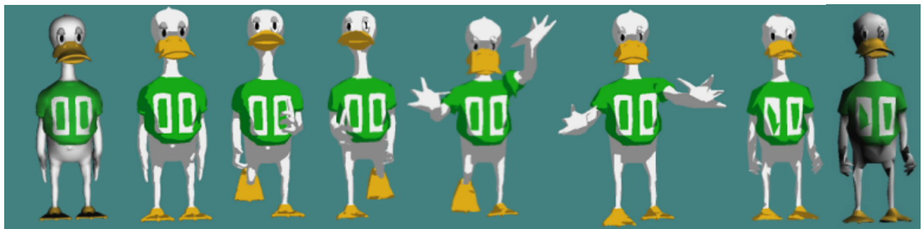
Figure 19: An example animation sequence that uses our cartoon shading technique and runs in real time on a PC. The left and right images are Gouraud shaded. From left to right the number of polygons was decreased at runtime to increase frame rate. The leftmost image has 16,000 polygons, and the rightmost has 1,000.
